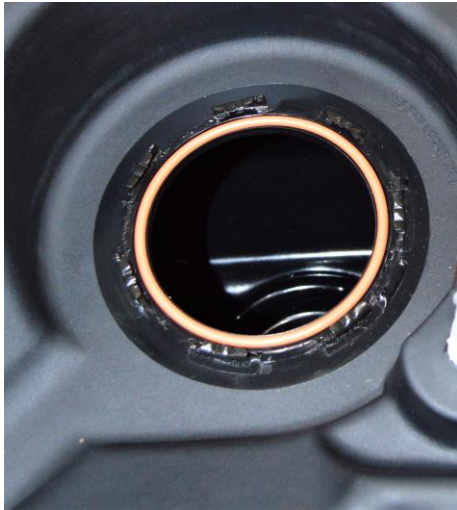
(Fig. 3) O-Ring gasket shown installed correctly.
