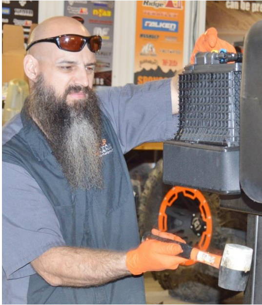
(Fig. 8) Using a rubber mallet, carefully tap the water separator up and out of its mounting bracket on the OEM tank.
