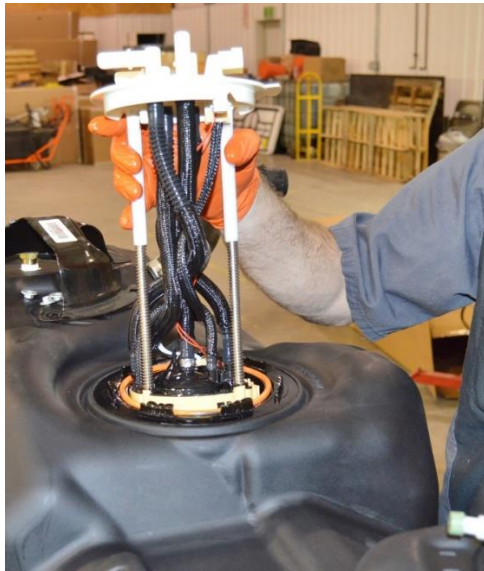
(Fig. 10) Place sending unit into the TITAN tank.
