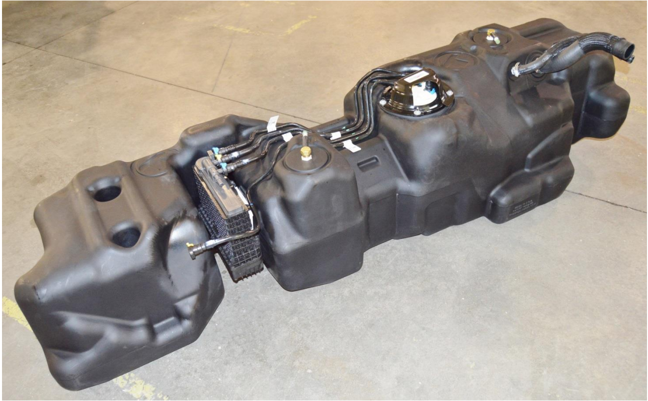
(Fig. 13) TITAN 7020217 tank shown with sending unit, water separator, fuel lines, sending unit guard, and fill and vent hoses installed; ready for installation into the vehicle.
