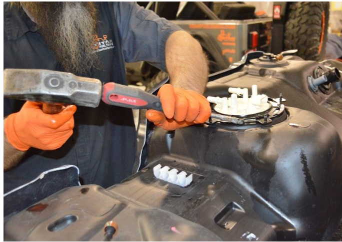
(Fig. 9) Loosen hold-down ring by turning it counter-clockwise as shown.
