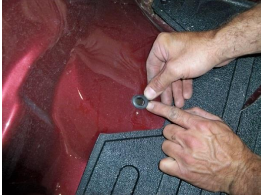
(Fig. 10) Install rubber grommet into fuel line hole(s).
