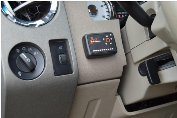
(Fig. 18) TITAN™ Electronic Controller mounted on dash.
