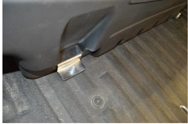
(Fig. 11) Toe clamps installed on Mounting Brackets
