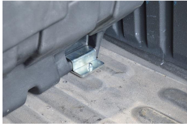
(Fig. 11) Toe clamps installed on Mounting Brackets
