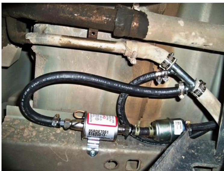
(Fig. 14) Under the vehicle, showing the Vent Line Filler Adapter installed in the vehicle's vent line.
