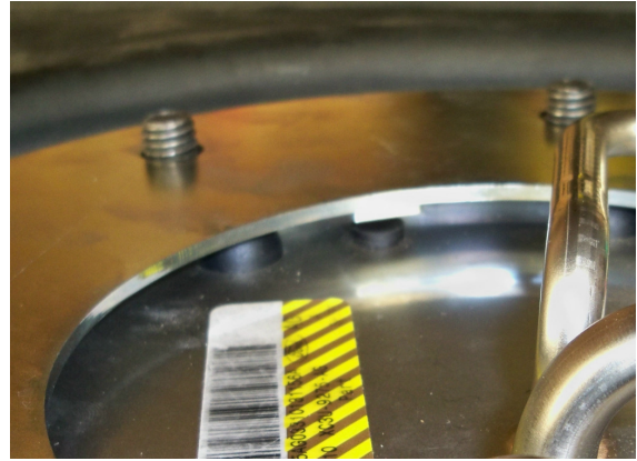
(Fig. 6b) Align tabs with small rubber plugs.
